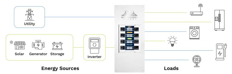
Typical installation showing SMART LOAD CENTER's Patented Dual Bus Architecture, sharing Utility to some loads and alternate energy to different loads simultaneously.
