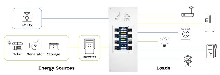
Typical installation showing SMART LOAD CENTER's Patented Dual Bus Architecture, sharing Utility to some loads and alternate energy to different loads simultaneously.
